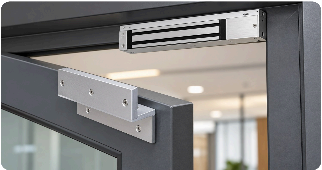
EM lock with Z + L bracket on a door that opens towards the lock.
